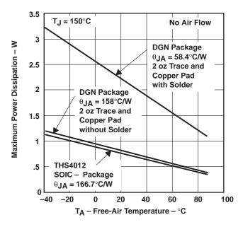
Even though the THS4012 EVM PCB is smaller than the one in the example above, the results should give an idea of how much power can be dissipated by the PowerPAD IC package. The THS4012 EVM is a good example of proper thermal management when using PowerPAD-mounted devices.
